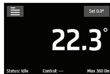
Fig. 1 Type 9640-A-001 touchscreen – displays the actual position of the platter. It is also used to set up various turntable parameters via softkeys
