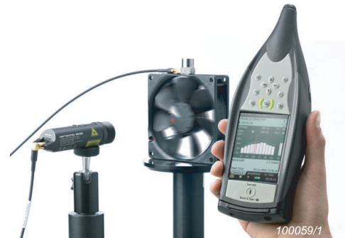
Fig. 3 Type 2981 with Integrating Hand-held Vibration Analyzer Type 2250-V for product vibration testing
