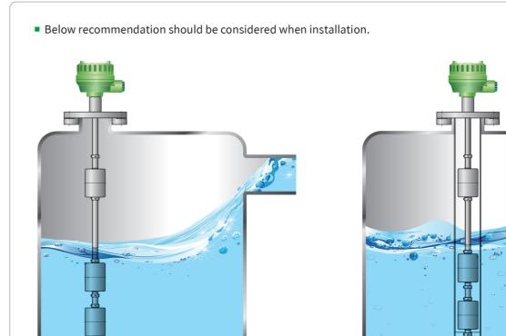
Product should be installed at the place far from inlet in order to avoid the malfunction.
