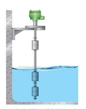
Bracket should be installed with the product when the installation on the concrete as per above figure.
