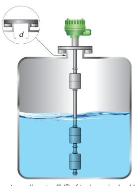
Inner diameter ("d") of tank nozzle should be larger than the outer diameter of float as per above figure.
